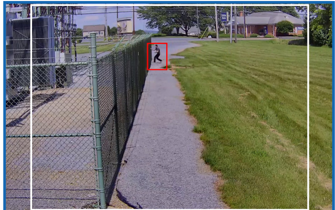
White border indicates thermal detection zone
