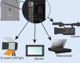
The D-Tap power output function is available from both D-Taps on IPI Series batteries
